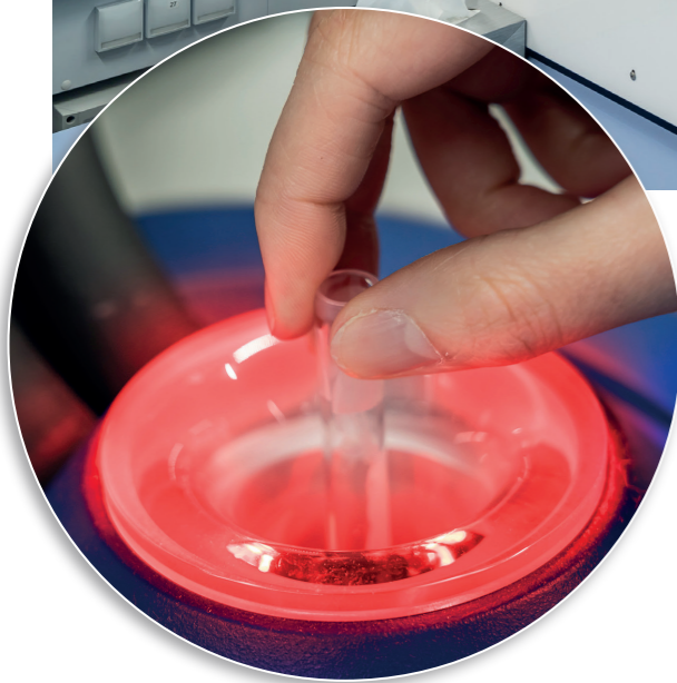
The new Bureau Veritas lab where solid fat content measurements are taken using a benchtop NMR analyser. The screen shows which steps need to be followed.
