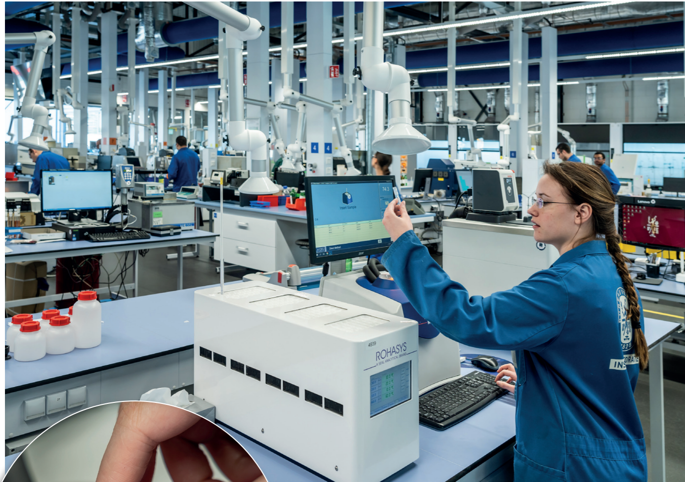
The new Bureau Veritas lab where solid fat content measurements are taken using a benchtop NMR analyser. The screen shows which steps need to be followed.
