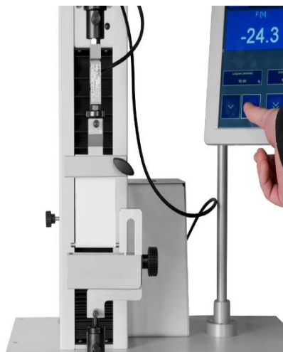
Wet tensile test acc. to FINCH
